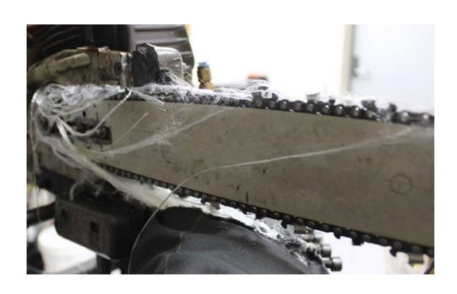
When a chainsaw chain hits this mat the teeth act like hooks, dragging these fibres out, which then get tangled around the sprocket, choking it.
